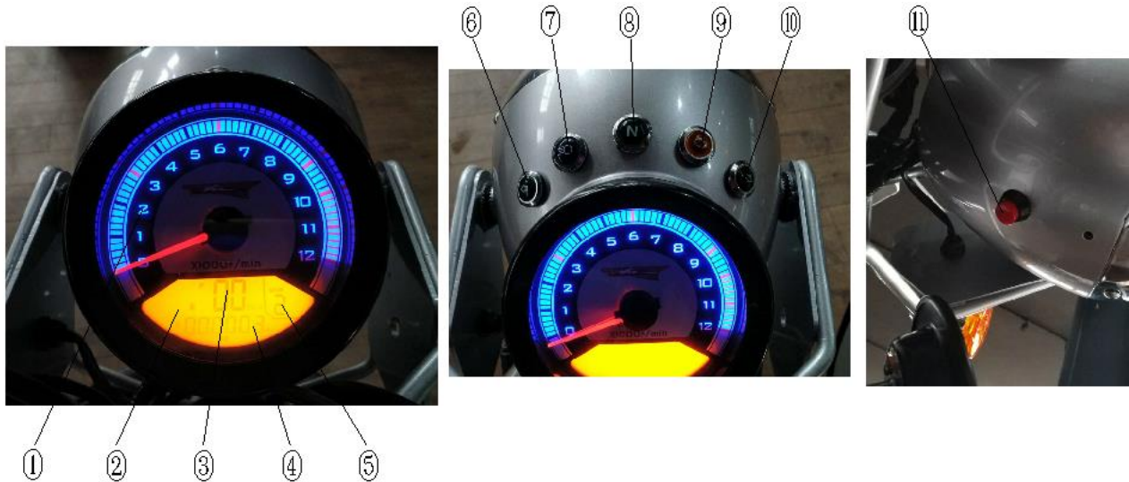
① Engine tachometer ②. Fuel gauge ③. Display of vehicle speed ④. Total mileage/mileage subtotal ⑤. Gear Display and Reverse R Display ⑥. Indicator light for left turn ⑦. High beam indicator light ⑧. Neutral gear indicator light. ⑨. diagnostic fault indicator light ⑩. Indicator light for right turn ⑪ Reset/ODO button.
