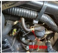
8) From this point the airbox can be removed by loosening the two clamps on the left and right rubber manifolds on the throttle body, and the engine breather hoses on the top left and the bottom of the airbox.
