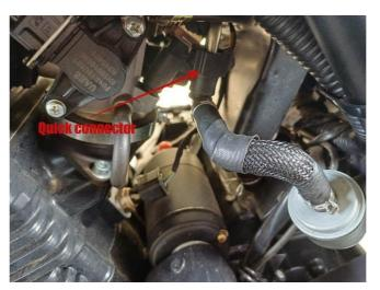
2) Using a quick connector coupling (commonly used on airline connectors), connect a length of fuel hose to the quick connector and into a fuel container. Switch the ignition on and cycle the kill switch on and off. Each time the kill switch is cycled fuel will be pumped out of the bottom tank. Usually 4-5 cycles are enough to drop the fuel level below that of the main tank.
