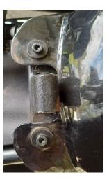
5) Remove the two screws holding the plastic frame shroud.
