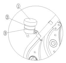
(1) Rear brake oil cup (2) upper limit scale line (3) lower limit scale line
