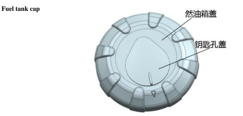
To open the fuel tank cap: turn the keyhole cover, insert the key and turn it clockwise. To lock the fuel tank cap: insert the key into the cap, and press the cap into the fuel. The key will automatically return to the box and can then be pulled out.
