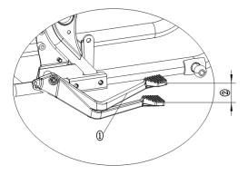
(1) Rear brake pedal (2) rear brake pedal stroke
