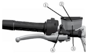
Check whether the brake fluid level in the front and rear brake oil cups is between the upper and lower scales.
