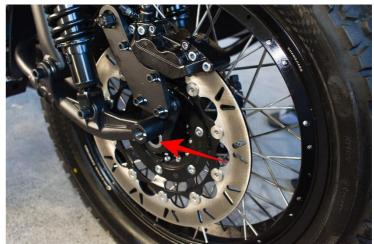
7) Lift the brake caliper upwards and roll the wheel forwards so that the brake caliper is free from the brake disc. Jack the wheel up higher as required to remove the wheel.
