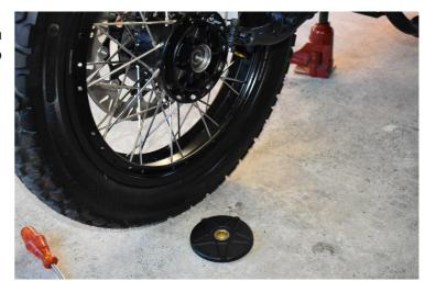
6) On the right side of the wheel, the brake caliper bracket will be loose as shown.
