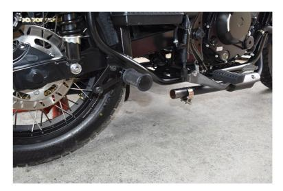
5) Loosen the chain adjusters on both left and right side of swingarm end (2 x 13mm spanners). Remove axle shaft splitpin and loosen 27mm axle nut. Push wheel forwards to create slack on the chain..
