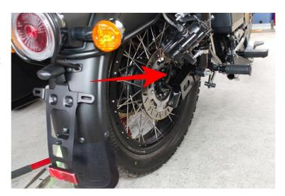
8) Take note of the way that the bracket is fitted. The locating slot must be located onto the swingarm when replacing.
