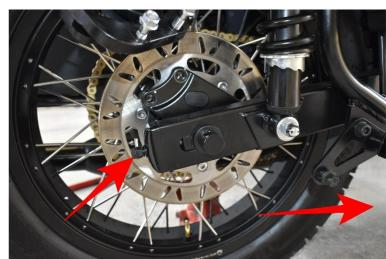
6) To prevent the chain sprocket and carrier dropping down use a strap to hold the sprocket in the same position when the axle shaft is removed.
