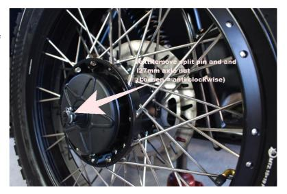
5) Slide the wheel outwards off the axle shaft.
