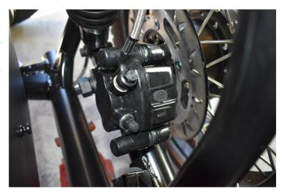
4) Jack the wheel up so that it is clear of the ground and remove the split pin and 27mm axle nut.
