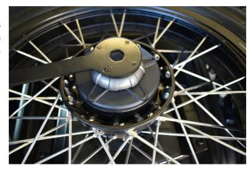
2) When the spare wheel is removed take note of the position of the locating pin recess in the carrier and the matching slot in the rubber cushion.
