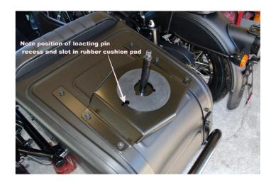
3) NB: take note of the locating pin screwed into the disc brake attaching bolt hole. This pin must be removed from the spare wheel and fitted to the wheel being put back on the sparewheel carrier. When refitting the wheel to the carrier ensure the pin is located in the spare wheel locating slot.
